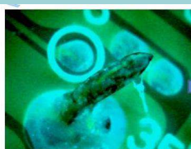
30μm film thickness on PCB surface
